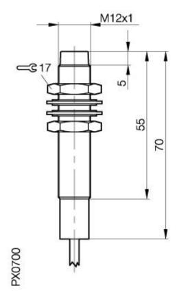
**Inductive Sensors** BES 113-356-SA 6-PU-03 M12x1 x 70 normally-open **Sn=3,7mm** unshielded function monitoring
